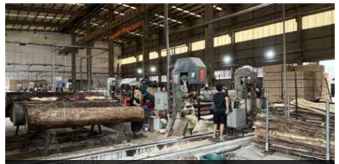
A typical Chinese sawmill unit working - the first stage of breaking down the log.
